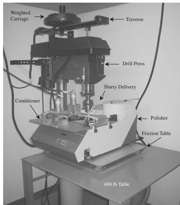
Fig. 1. Scaled polisher showing the diamond disc conditioner, the drill press and the traverse assembly.
