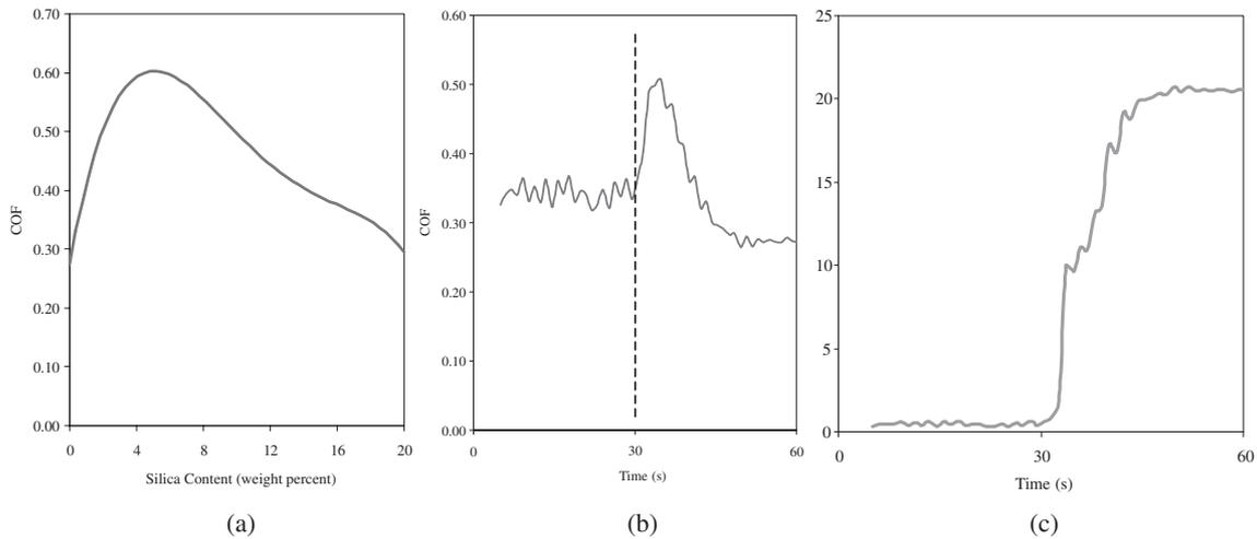
Fig. 5. COF as a function of Syton-OXK colloidal silica slurry solids concentration (a); actual response (COF versus time) corresponding to 20% weight percent Syton-OXK slurry displacing water during a polish process (b); corresponding silica concentration response (c).
