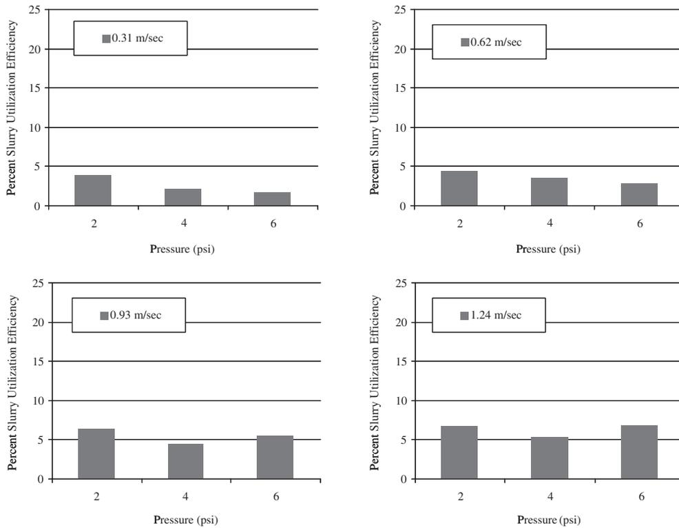
Fig. 7. Slurry utilization efficiency as a function of pressure, velocity and slurry flow rate for Phase II studies.
