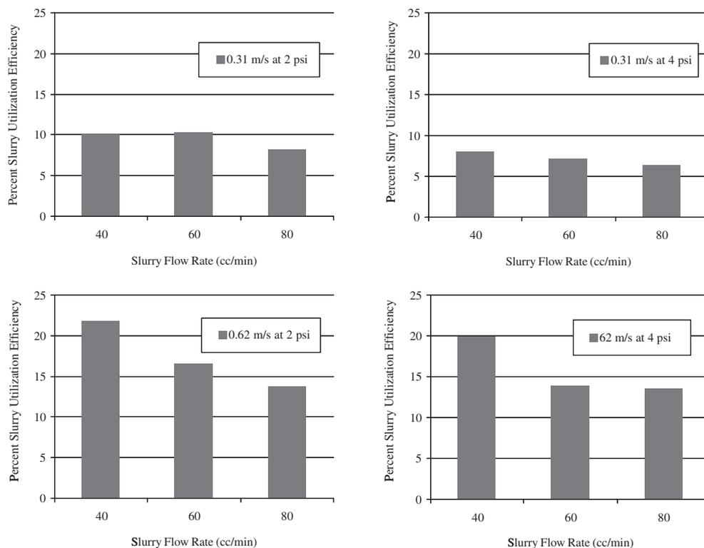
Fig. 6. Slurry utilization efficiency as a function of pressure, velocity and slurry flow rate for Phase I studies.
