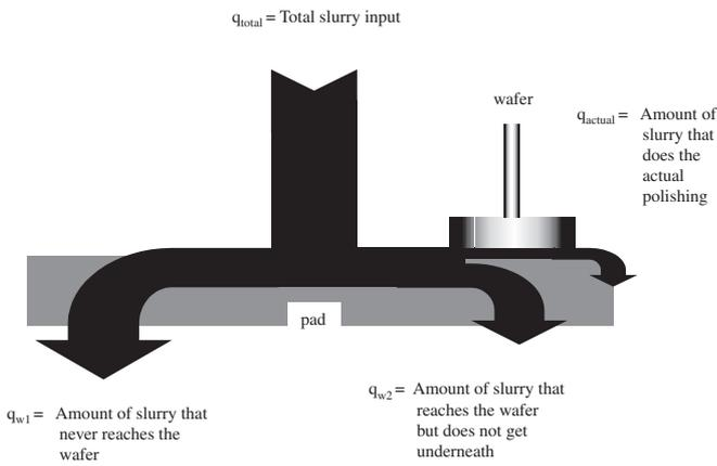
Fig. 2. Various paths the fluid can take during CMP.
