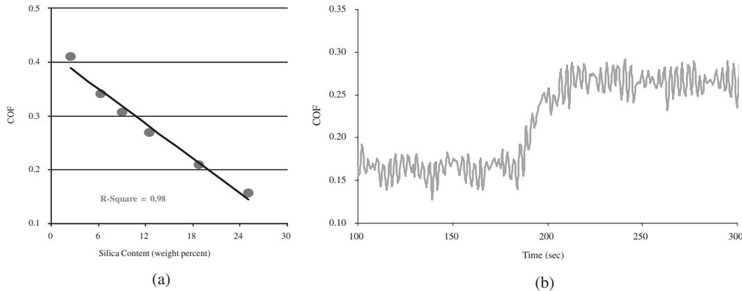
Fig. 3. Relationship between COF and silica concentration (a) and the resulting F-curve (b).
