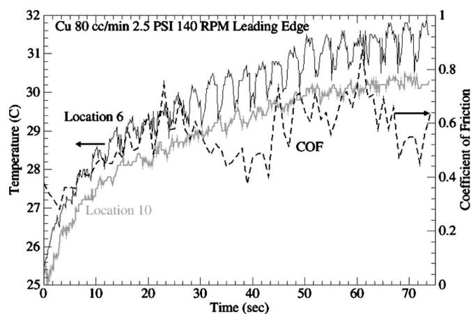
**Figure 2.** Pad temperatures at sample points 6 and 10 and the measured COF at 2.5 psi/140 rpm, 80 cm<sup>3</sup>/min.
