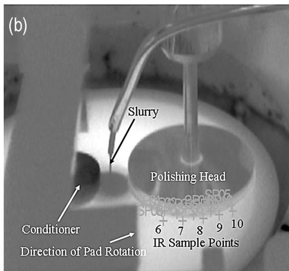
**Figure 1.** (a) Image of scaled polisher showing the diamond disk conditioner, drill press, and friction table. (b) Locations of leading edge sample points at which thermal data were measured.
