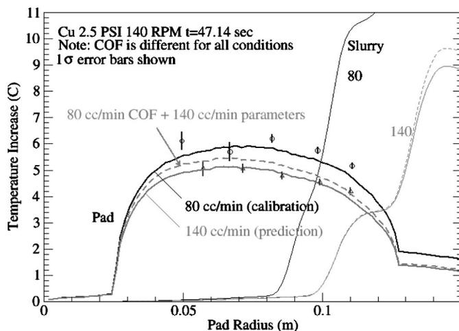
**Figure 7.** Simulated (solid curves) and measured (points with error bars) pad and slurry temperatures at 80 and 140 cm<sup>3</sup>/min slurry flow rates along a radial line running approximately through sample points 6-10. Also shown are the slurry temperature distributions and a curve that suggests the relative influences of the COF and the pad-slurry heat-transfer coefficient.
