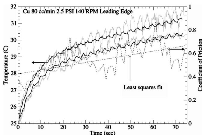
**Figure 6.** Measured (light solid curves) and simulated (dark solid curves) pad temperatures at pad locations 6 and 10 at 80 cm<sup>3</sup>/min flow rate. Also shown is the measured COF and the linear regression to the COF that was used in the simulations.
