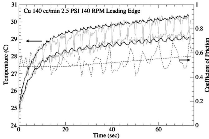
**Figure 3.** Measured (light solid curves) and simulated (dark solid curves) pad temperatures at pad locations 6 and 10 at 140 cm<sup>3</sup>/min flow rate.
