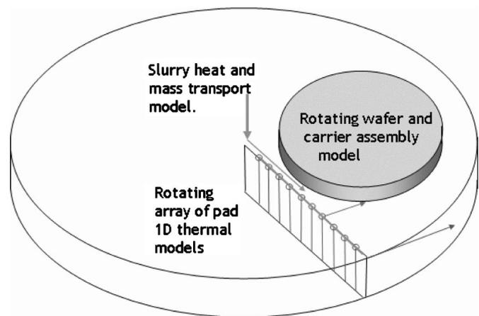
**Figure 5.** Schematic of the numerical approach in Ref. 5 for simulating heat-transfer in a rotary CMP tool.
