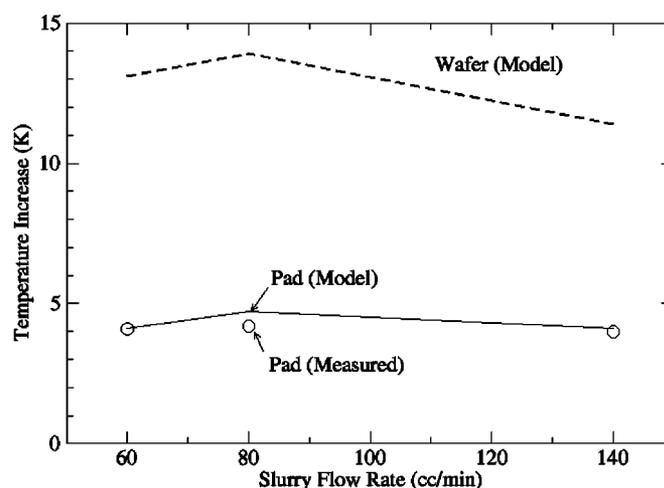
**Figure 8.** Comparison of overall mean (—) calculated and (○) measured pad temperature increase at sample points 6-10 vs. flow rate. (---) The calculated mean wafer temperature increase.
