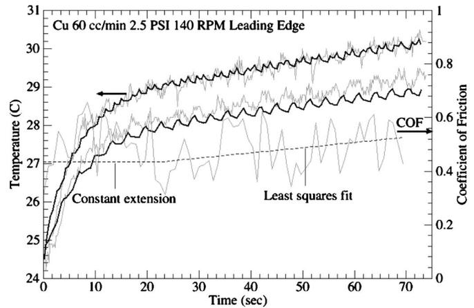
**Figure 4.** Measured (light solid curves) and simulated (dark solid curves) pad temperatures at pad locations 6 and 10 at 60 cm<sup>3</sup>/min flow rate.
