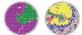
Fig. 2: Keyhole patterns detected at final wafer sort.
