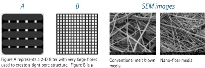
Figure A represents a 2-D filter with very large fibers used to create a tight pore structure. Figure B is a filter of similar pore size, but utilizing much smaller fibers. The smaller fibers allow for many more pores which greatly improves the flow performance, while maintaining the tight pore structure.
